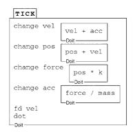
Figure 8. Ned and Dave's tick procedure for the Spring simulation.
